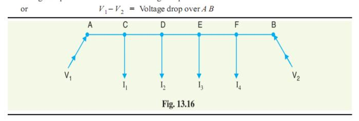
**Example 13.10.** A 2-wire d.c. street mains AB, 600 m long is fed from both ends at 220 V. Loads of 20 A, 40 A, 50 A and 30 A are tapped at distances of 100m, 250m, 400m and 500 m from the end A respectively. If the area of X-section of distributor conductor is  $1 \text{ cm}^2$ , find the minimum consumer voltage. Take  $\rho = 1.7 \times 10^{-6} \Omega \text{ cm}$ .
