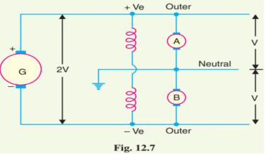
erator and supplies power to the whole system. The balancer set consists of two identical d.c shunt machines *A* and *B* coupled mechanically with their armatures and field windings joined in series across the outers. The junction of their armatures is earthed and neutral wire is taken out from here. The balancer set has the additional advantage that it maintains the potential difference on two sides of neutral equal to each other. This method is discussed in detail in the next chapter.
