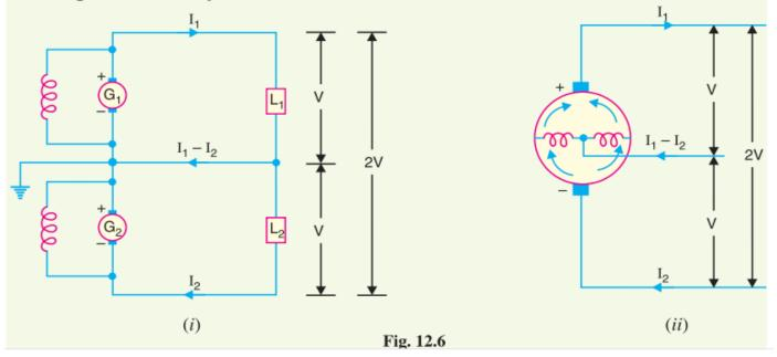
(ii) 3-wire d.c. generator. The above method is costly on account of the necessity of two gen-
