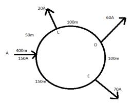
36. A 300m ring distributor has loads as shown in figure, where distances are in meters. The resistance of each conductor is  $0.2\Omega$  per Km and the loads are tapped off at points B, C and D as shown. If the distributor is fed at A at 240V, find voltages at B, C and D.
