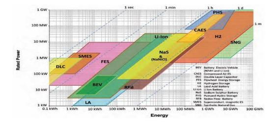
Lead Acid - Lead acid batteries are the world's most widely used battery type and have been commercially deployed since about 1890. Their usability decreases when high power is discharged and this makes them unviable as MW scale solutions.
