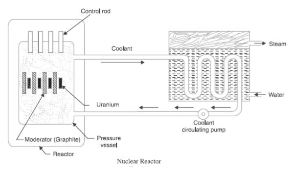
(ii) Heat exchanger: The coolant gives up heat to the heat exchanger which is utilized in raising the steam. After giving up heat, the coolant is again fed to the reactor.
