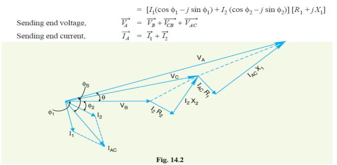
The vector diagram of the a.c. distributor under these conditions is shown in Fig. 14.2. Here, the receiving end voltage  $V_B$  is taken as the reference vector. As power factors of loads are given *w.r.t.*  $V_B$ , therefore,  $I_1$  and  $I_2$  lag behind  $V_B$  by  $\phi_1$  and  $\phi_2$  respectively.
