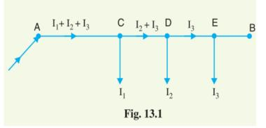
*distributor*) and loads  $I_1$ ,  $I_2$  and  $I_3$  tapped off at points C, D and E respectively.
