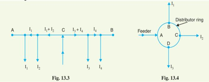
(iv) Ring mains. In this type, the distributor is in the form of a closed ring as shown in Fig.13.4. It is equivalent to a straight distributor fed at both ends with equal voltages, the two ends being brought together to form a closed ring. The distributor ring may be fed at one or more than one point.
