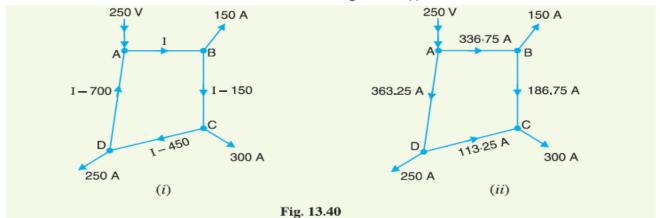
According to Kirchhoff's voltage law, the voltage drop in the closed loop ABCDA is zero i.e.
