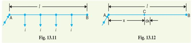
Consider a point C on the distributor at a distance x metres from the feeding point A as shown in Fig. 13.12. Then current at point C is
