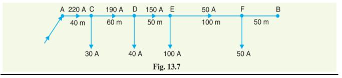
Referring to Fig. 13.7, the currents in the various sections of the distributor are :
