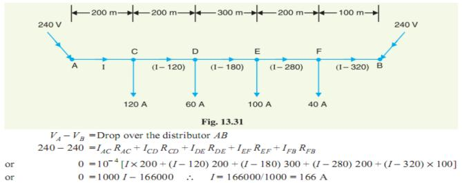
The actual distribution of currents in the various sections of the distributor due to concentrated loading is shown in Fig. 13.32. It is clear from this figure that *D* is the point of minimum potential.
