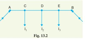
on decreasing as we move away from one feeding point say A, reaches minimum value and then again starts rising and reaches maximum value when we reach the other feeding point B. The minimum voltage occurs at some load point and is never fixed. It is shifted with the variation of load on different sections of the distributor.
