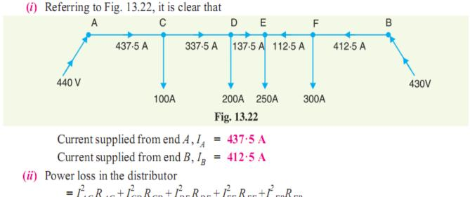
$$= I_{AC}^{2} R_{AC} + I_{CD}^{2} R_{CD} + I_{DE}^{2} R_{DE} + I_{EF}^{2} R_{EF} + I_{FB}^{2} R_{FB}$$
