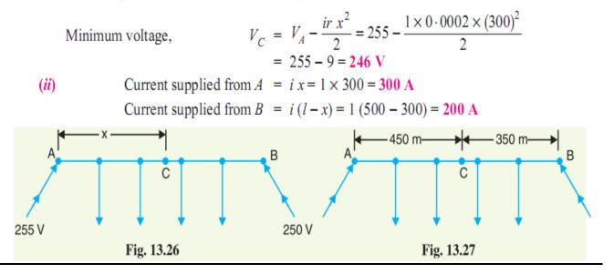
**Example 13.16.** A 800 metres 2-wire d.c. distributor AB fed from both ends is uniformly loaded at the rate of 1.25 A/metre run. Calculate the voltage at the feeding points A and B if the minimum potential of 220 V occurs at point C at a distance of 450 metres from the end A. Resistance of each conductor is  $0.05 \Omega/km$ .
