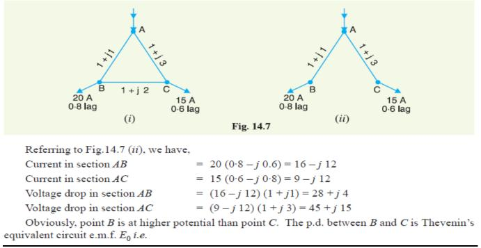
The venin's equivalent circuit e.m.f.,  $E_0 = p.d.$  between B and C =  $(45 + j \ 15) - (28 + j \ 4) = 17 + j \ 11$
