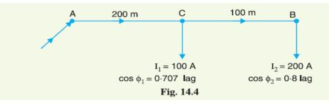
Impedance of section AC,  $\overrightarrow{Z_{AC}} = (0.2 + j \ 0.1) \times 200/1000 = (0.04 + j \ 0.02) \Omega$ Impedance of section CB,  $\overrightarrow{Z_{CB}} = (0.2 + j \ 0.1) \times 100/1000 = (0.02 + j \ 0.01) \Omega$ Taking voltage at the far end B as the reference vector, we have,
