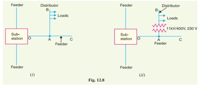
This is the simplest distribution circuit and has the lowest initial cost. However, it suffers from the following drawbacks :
