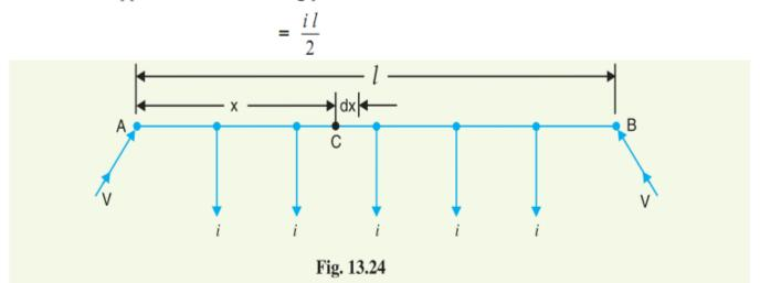
Consider a point C at a distance x metres from the feeding point A. Then current at point C is
