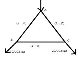
61. A 3-phase, 6.6 KV sub-station supplies a load of 120A at 0.8 p.f lagging at B and 75A 0.6 p.f lagging at C. the impedance of each branch is shown in figure. Find out the current in each branch, the p.f of load are referred to the section A.
