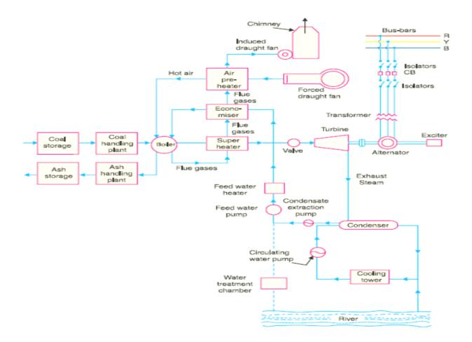
Although steam power station, simply involves the conversion of heat of coal conversion into electrical energy, yet it embraces many arrangements of proper working an efficiency.
