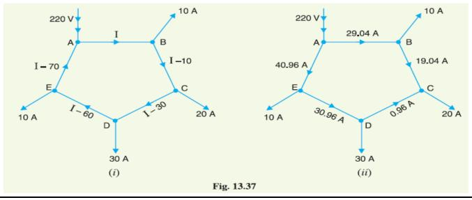
(i) According to Kirchhoff's voltage law, the voltage drop in the closed loop *ABCDEA* is zero *i.e.*  $I_{AB} R_{AB} + I_{BC} R_{BC} + I_{CD} R_{CD} + I_{DE} R_{DE} + I_{EA} R_{EA} = 0$
